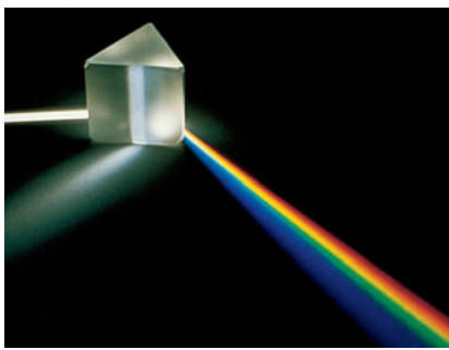
FIGURE 24-13 White light passing through a prism is spread out into its constituent colors.
