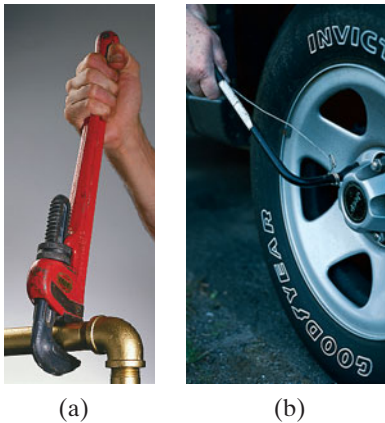
FIGURE 8-11 (a) A plumber can exert greater torque using a wrench with a long lever arm. (b) A tire iron too can have a long lever arm.
