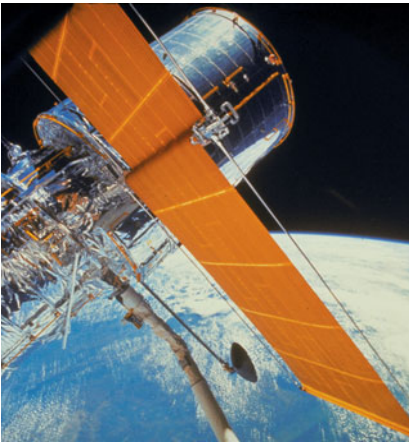
FIGURE 25–32 Hubble Space Telescope, with Earth in the background. The flat orange panels are solar cells that collect energy from the Sun to power the equipment.
