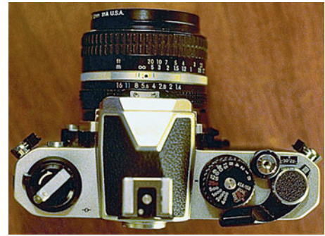
FIGURE 25–5 On this camera, the f -stops and the focusing ring are on the camera lens. Shutter speeds are selected on the small wheel on top of the camera body.
