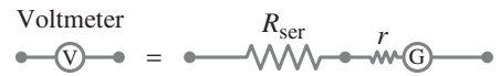
FIGURE 19–32 A voltmeter is a galvanometer in series with a resistor with high resistance, R_{\text{ser}} .
