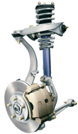
FIGURE 11-4 Photo of a car's spring. (Also visible is the shock absorber, in blue—see Section 11-5.)
