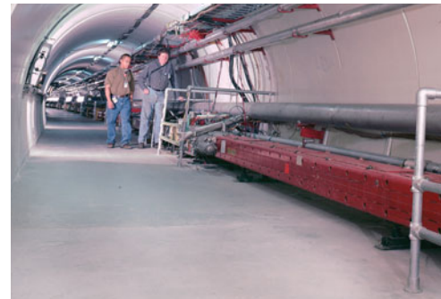
FIGURE 32–3 The interior of the tunnel of the main accelerator at Fermilab, showing (red) the ring of superconducting magnets used to keep particles moving in a circular path at the 1-TeV Tevatron.
